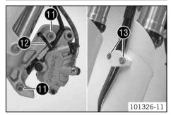
Position the brake caliper. Mount and tighten screws ①.
