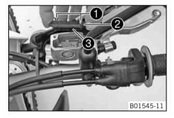
Move the brake fluid reservoir mounted on the handlebar to a horizontal position.
