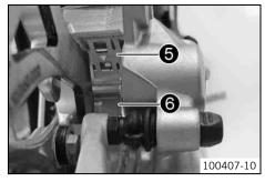
Check that leaf spring **6** in the brake caliper and sliding plate **6** in the brake caliper support are seated correctly.
