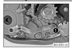
The engine number  $oldsymbol{0}$  is stamped on the left side of the engine under the engine sprocket.
