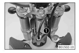
Press release button •, turn filler cap counterclockwise and lift it upwards and remove.
