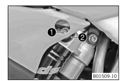
Turn adjusting screw • clockwise with a screwdriver up to the last perceptible click.
