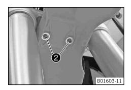
Mount and tighten screws ②.
