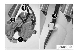
Position the brake caliper and mount and tighten screws 4.
