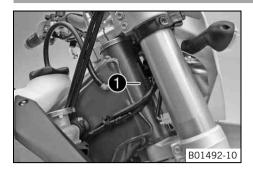
The chassis number • is stamped on the steering head on the right.
