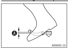
Sit on the vehicle in the riding position and determine the distance between the upper edge of your boot and the shift lever.
