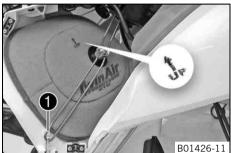
Insert both parts together, position them and fasten them using air filter holder ①. The arrow of marking **UP** faces up.
