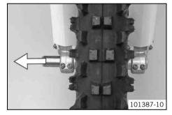
Holding the front wheel, withdraw the wheel spindle. Take the front wheel out of the fork.
