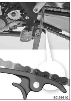
Pull on the upper part of the chain with the specified weight **a**.
