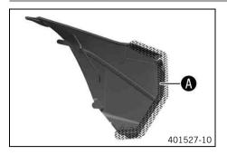
Seal the air filter box in the marked area **A**.
