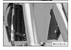
Pull both spoilers off of the sides of the radiator bracket and lift off the fuel tank.
