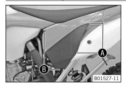
– Insert the air filter box lid into the rear area  $oldsymbol{0}$  and clip it into the front area  $oldsymbol{0}$ .
