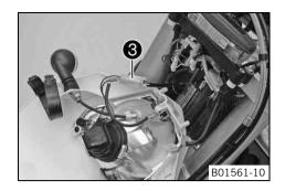
Pull out the electric plug connector 3 and remove the headlight mask with the headlight.
