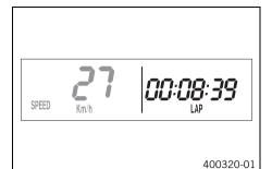
In the LAP display mode, up to 10 lap times can be timed with the stop watch.
