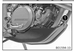
Turn quick release • counterclockwise until it disengages. Remove the engine guard.
