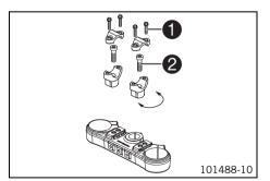
Remove the four screws ①. Remove the handlebar clamps. Remove the handlebar and lay it to one side.
