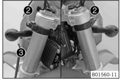
Position the headlight mask and fix it with the rubber band ②.
