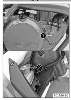
Water pump **1** in the engine circulates the coolant.
