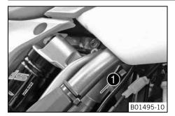
The shock absorber part number  $\pmb{\bullet}$  is stamped on the top of the shock absorber above the adjusting ring on the engine side.
