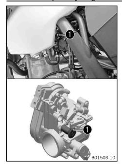
The idle speed adjusting screw **1** is located on the throttle valve body at the top left. The idle speed adjusting screw has two functions.
