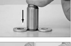
If you press the timing chain tensioner again and it extends no more than half way (preventing it from extending completely), the stop system will lock and the timing chain tensioner can no longer be pressed together - this position is necessary to ensure that the timing chain is adequately tensioned, even if the oil pressure is low.
