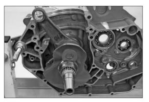
Simultaneously remove both transmission shafts from the engine \_ case half.
