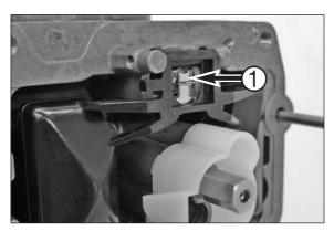
If the float needle valve is good you can adjust the float height by bending the float tab ①.
