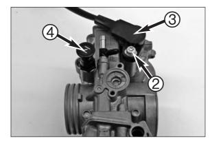
NOTE: only remove the throttle sensor if it is defective. If you loosen the screw @, you will need to readjust the throttle sensor.
