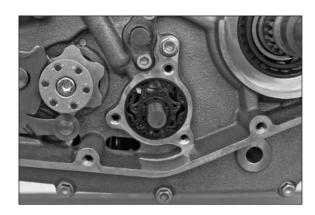
Remove the suction oil pump together with the oil pump shaft and \_ needle roller.
