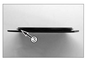
Check the membrane ③ on the throttle slide plate for cracks or brittleness and make sure it is correctly seated.
