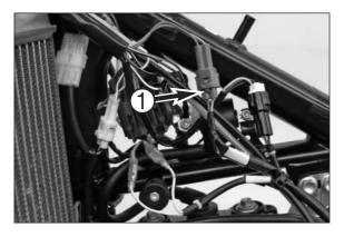
**Check the pickup** for an output signal - bipolar plug **1** with green and red cable colors (also see circuit diagram on page 7-6):
