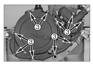
Remove the screws ③ and completely take off the clutch cover. \_
