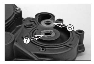
Pry out the water pump shaft seal rings
