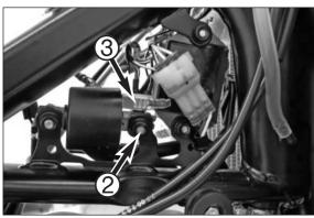
**Check the primary voltage for ignition coil control** (also see circuit diagram on page 7-6) for voltage (blue/white cable):
