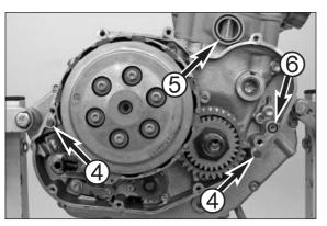
Pull the rollers ④ out of the engine case. Remove the quad ring ⑤ and O-ring ⑥. \_
