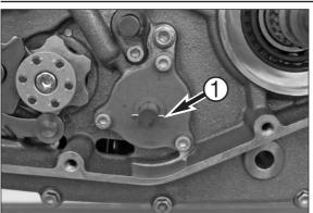
\_ Remove the needle roller ①.
