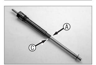
Insert the market jet needle in the needle jet to be tested. **Carefully** push the two parts together. If the mark ④ on the jet needle can still be seen on the upper edge ④ of the needle jet, the needle jet can still be used.
