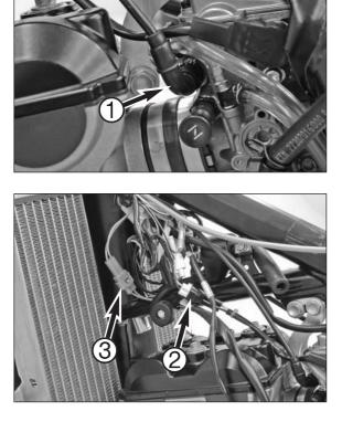
Connect the socket connectors on the throttle position sensor 2, pulse generator 3 and generator. Fasten the wiring harnesses with cable ties.
