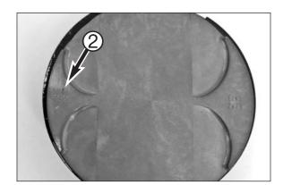
NOTE: The cylinder size ① is marked on the cylinder collar, the piston size ② on the piston head.
