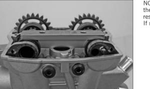
NOTE: if the camshaft gears were not pressed off the camshafts, check the adjusting bearing bridge 773.29.050.000. Its entire surface must rest against the cylinder head and the flat sides against the camshaft. If not, press off the camshaft gears and readjust.
