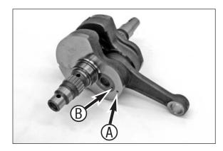
CAUTION IF THE CRANKPIN IS INSERTED IN THE WRONG POSITION, THE CONROD BEARING WILL NOT BE LUBRICATED WITH ENGINE OIL AND CAUSE THE BEARING TO BE DAMAGED.
