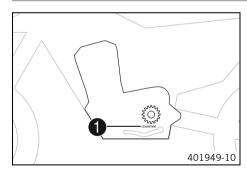
The engine number 1 is stamped on the left side of the engine under the engine sprocket.
