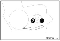
Remove screw with the washers and take off shift lever lever .
