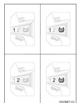
The combination switch displays the current drive mode and traction control setting.
