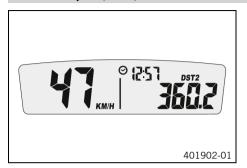
Press one of the buttons until **DST2** appears on the combination instrument.
