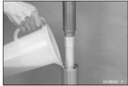
Raise the outer tube [A] and temporarily tighten the fork top plug (subtank) [B].
