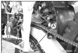
Visually inspect the chain slipper [A] on the swingarm and replace it if worn or damaged.
