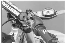
The torque of fork top plug is specified to **30 N-m** (**3.0 kgf-m**, **22 ft-lb**) however, when you use the top plug wrench (special tool) [A], reduce the torque to 90% of the specified value [**27 N-m** (**2.8 kgf-m**, **20 ft-lb**)] due to the distance [B] between the center of the square hole, where the torque wrench is fitted, and that of the octagonal hole of the wrench.
