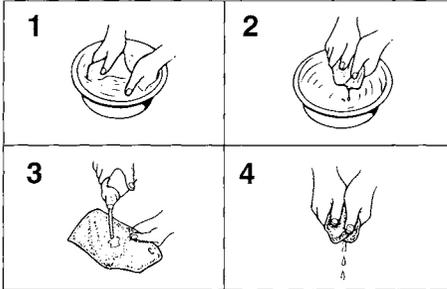
5. Clean the sponge material with solvent, and then squeeze the remaining solvent out.
