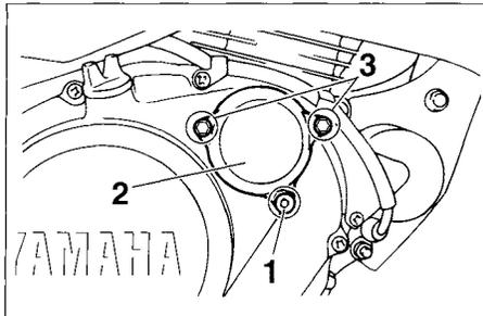
1. Oil filter element drain bolt
