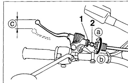
1. Locknut (clutch lever)
