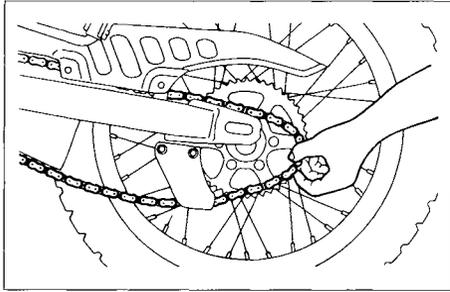
7. Push the wheel forward, and then remove the drive chain from the rear sprocket.
